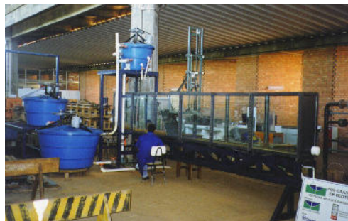
Fine Fraction Filtration Test – F 3 Test
